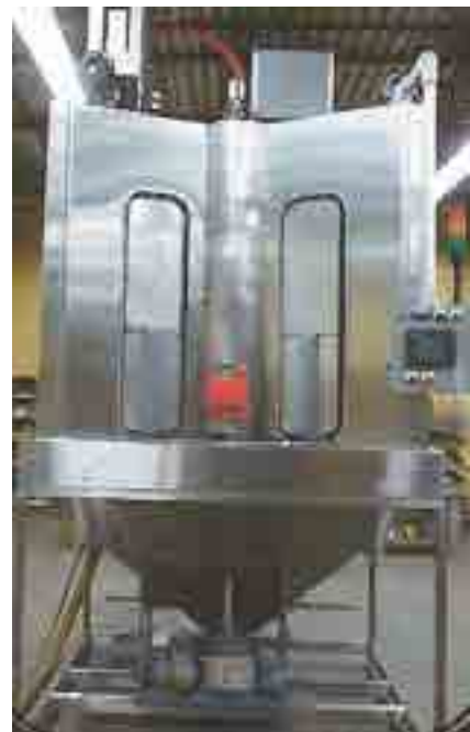
MEDIA BLASTING - MANUAL WET BLAST CABINET
